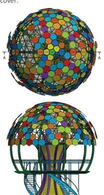
It took more than 400 specialist engineering manhours to design and develop the concept design into a workable model that could be constructed. A huge canopy layered with complex hexagons; intricate geometric mathematics and multiple 3D programs were utilised to create a roof structure capable of incorporating the hexagons, curved bars and node connections required to bear the structural and water loads of the completed raintrees.
